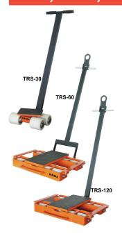
Nylon rollers running on bearings except for models TRS-120 fitted with steel rollers. Nylon rollers will not damage floors. Platforms have anti-slip rubber coatings. Can be easily placed or positioned by means of the hand grip.
